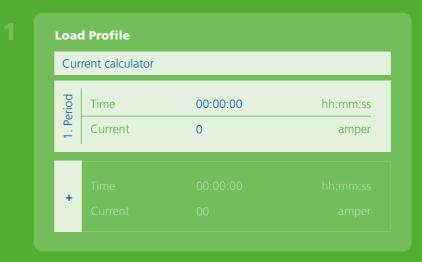
Through a guided User-Interface, fill in the basic parameters of the required or expected load the batteries will be handling for a specific application.
